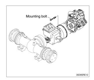
② Using a moving truck slowly pull out transmission assembly to the front.
