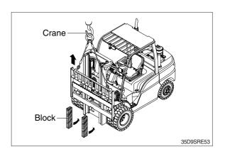
② While supporting lift chains, remove the split pin and nuts from the anchor bolt.
